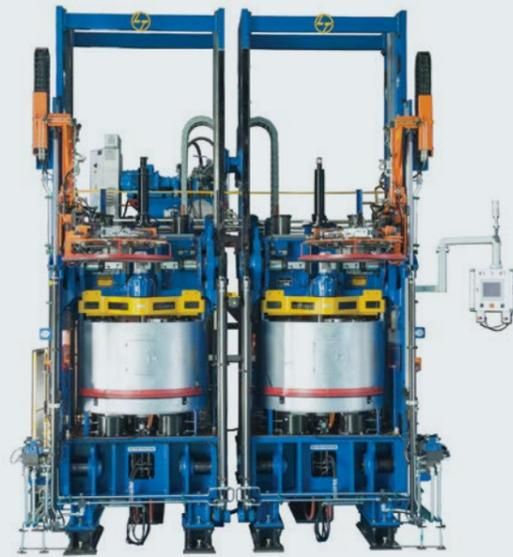
Truck Bus Hydraulic Tyre Curing Press
