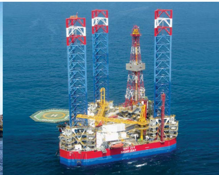
ONGC's jack-up rig 'Sagar Uday' (BMC Class 300) involving major lay-up and repair
