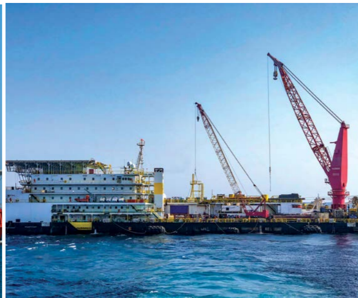
Marine services cover the entire spectrum of offshore installations - LTS 3000 (left), a heavy-lift-cum-pipelay vessel and LTB 300 (right), a pipelay-cum-work barge
