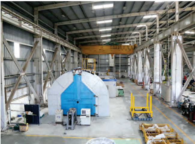
Regulating test bed at Howden's Hosur facility
