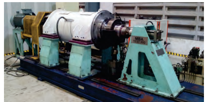
Main bearing assembly test bed at L&T Howden's Hazira facility
