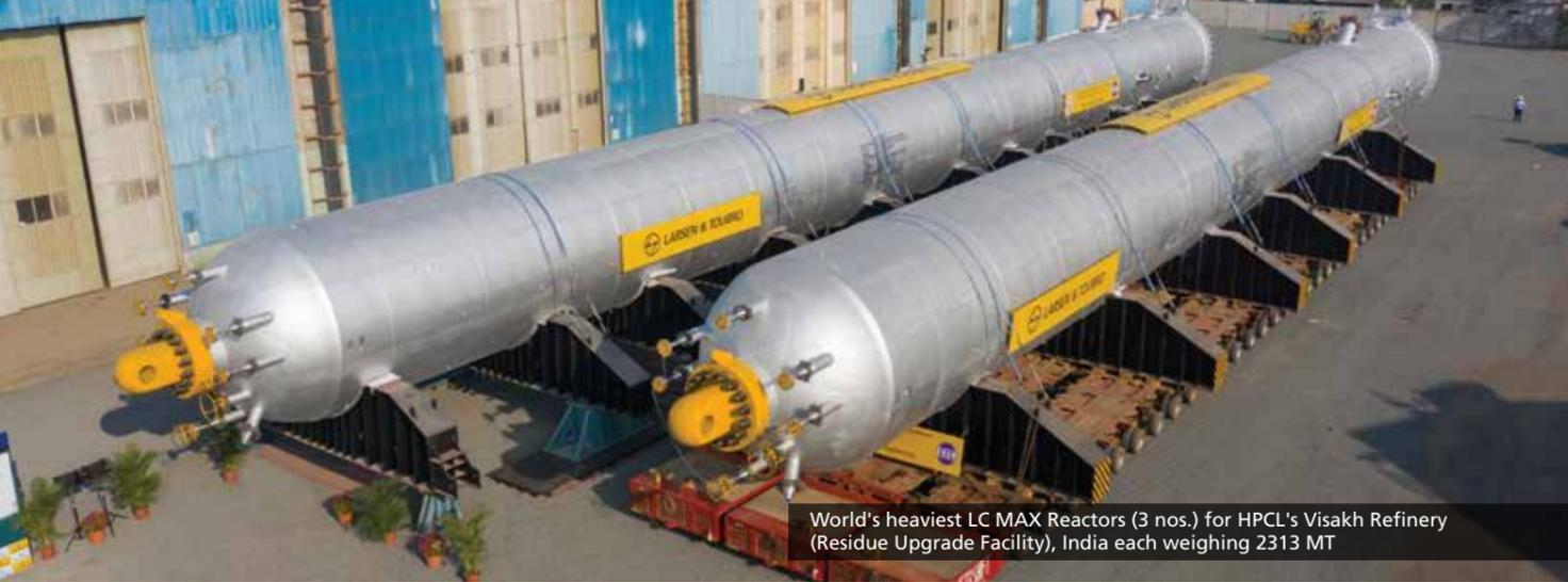
World's heaviest LC MAX Reactors (3 nos.) for HPCL's Visakh Refinery (Residue Upgrade Facility), India each weighing 2313 MT
