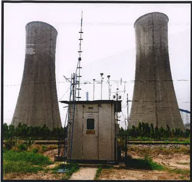
Pic-1 Four numbers of Continuous Ambient Air Quality Monitoring stations (CAAQMS) inside the plant to monitor ambient air quality.
