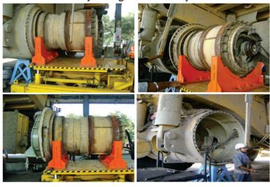
Fitment of Wheel Motor by using Wheel Motor Dolly
