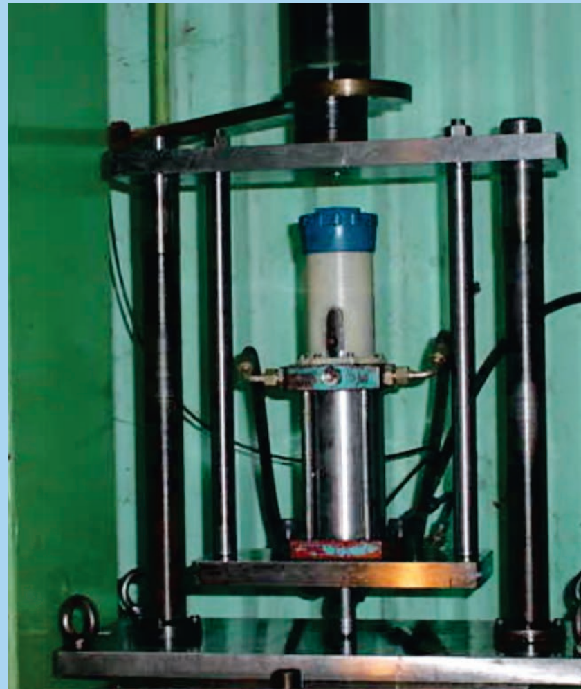
3.5 TON JACK UNDER TESTING
