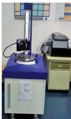
Form tester for Roundness Cylindricity, Straightness of super finished parts
