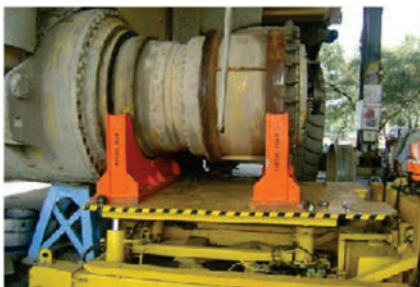
Removal and Fitment of Dump Truck Wheel Motor using Variable Work Table
