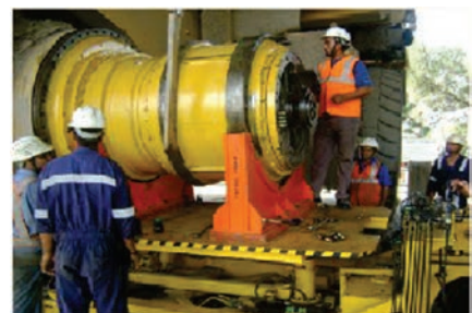
Removal and Fitment of Dump Truck Wheel Motor using Variable Work Table
