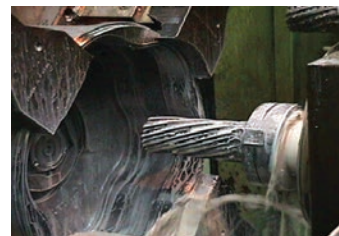
Hydraulics Motor Cam Profile machined on CNC m/c
