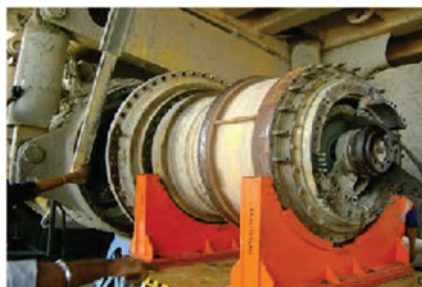
Removal and Fitment of Dump Truck Wheel Motor using Variable Work Table
