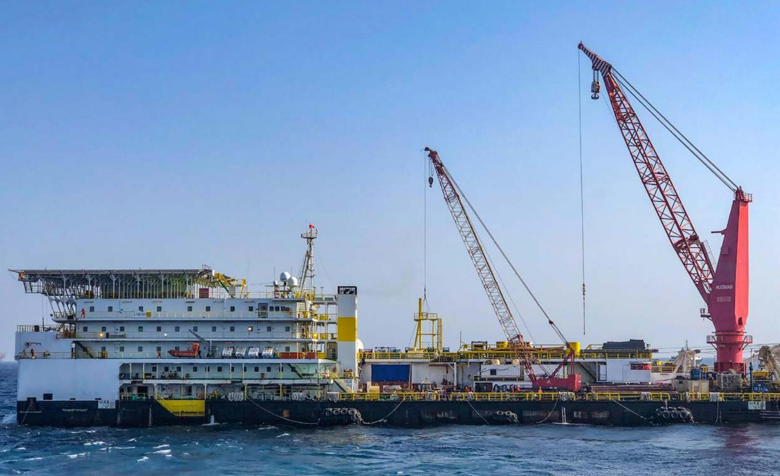
*LTB 300, a pipelay-cum-work barge undertaking offshore installation*
