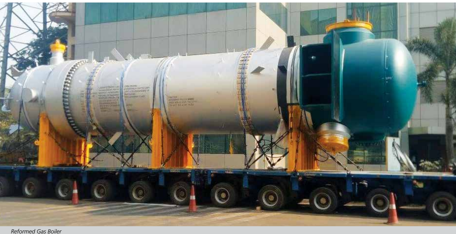
Reformed Gas Boiler
