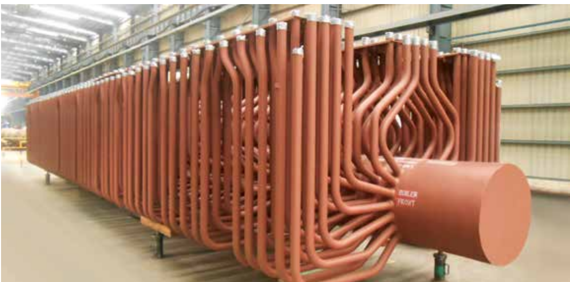
Boiler internals being manufactured at Hazira, Gujarat
