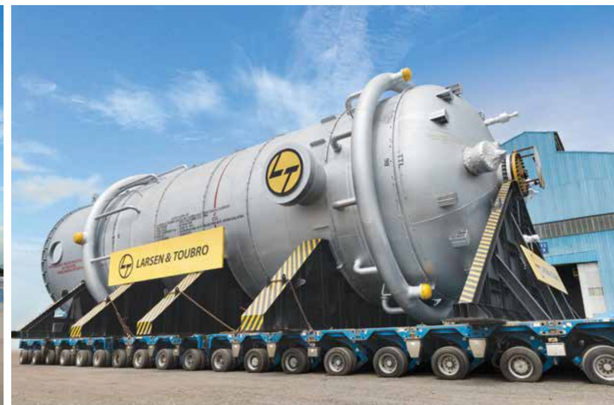
Ethylene Oxide Reactor
