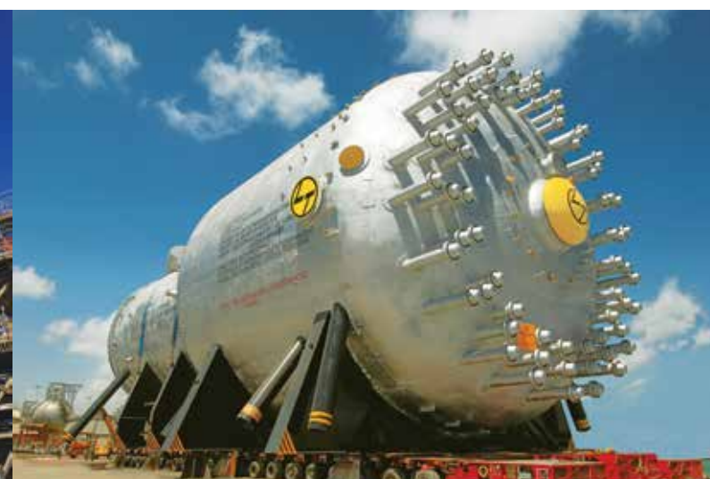
FCC Reactor & Regenerator
