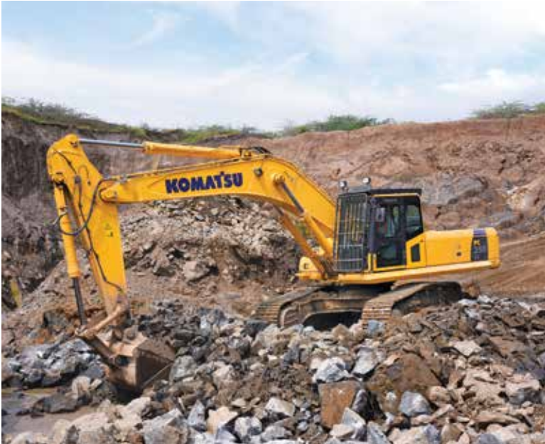
Komatsu PC350LC-8M0 Hydraulic Excavator
