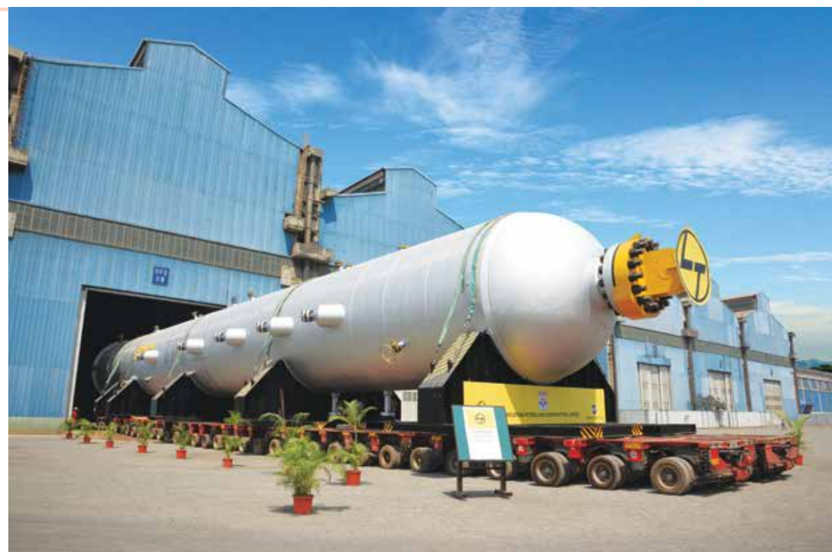
India's heaviest Hydrocracking Reactor (1858 MT)
