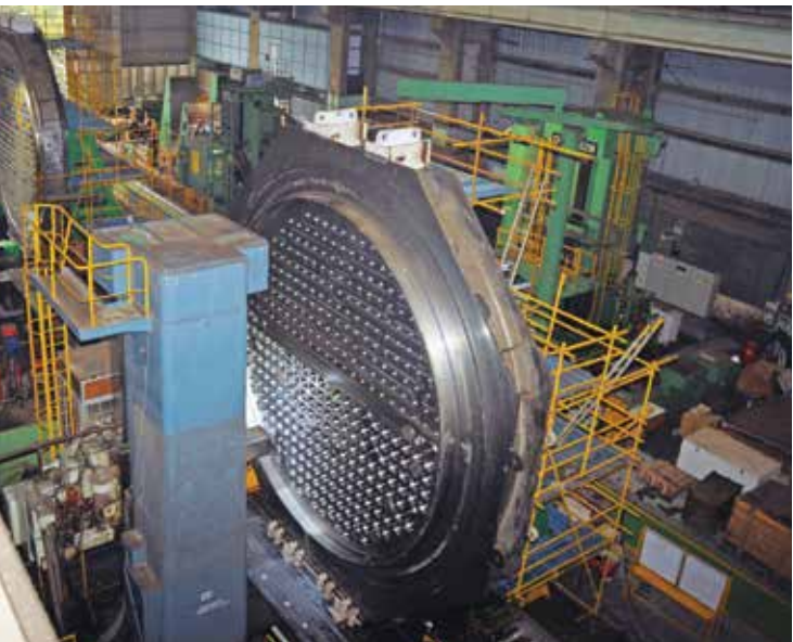
End-shields under manufacture
