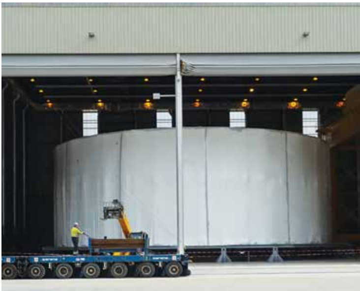
Lower Cylinder of Cryostat for ITER
