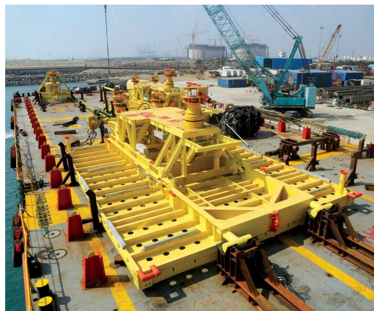
Loadout of subsea structure for ONGC's S1 Vashishta Deepwater Project from Kattupalli Facility
