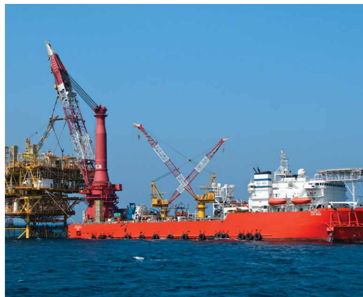
Marine services cover the entire spectrum of offshore installations - LTS 3000 (left), a heavy-lift-cum-pipeline vessel and LTB 300 (right), a pipeline-cum-work barge
