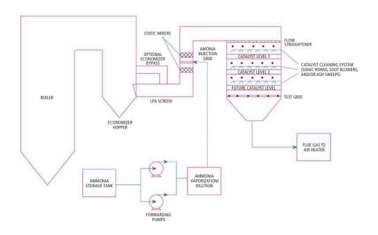
SCR is a capital-cost-intensive, post-combustion technology that uses catalyst elements installed in the flue gas stream upstream from the air-preheater to promote the  $NO_x$  reduction reaction.
