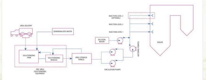
The SNCR process requires injection of urea into the flue gas within a temperature window of 1870-1090  $^{\circ}$ C to reduce NO<sub>x</sub> to nitrogen and water.
