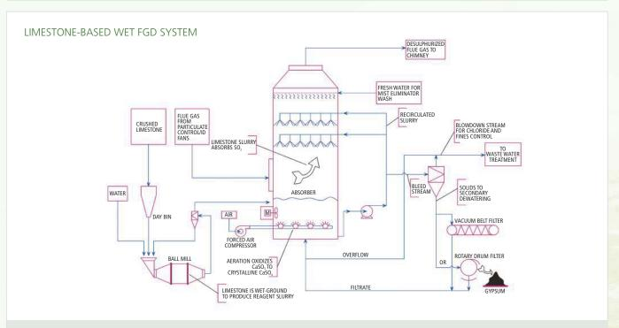
• Can accept a wide variety of fuel sulphur levels • Highly efficient at removing SO<sub>2</sub> and other acid gases • Can reduce mercury emissions • Can produce a saleable byproduct (gypsum)
