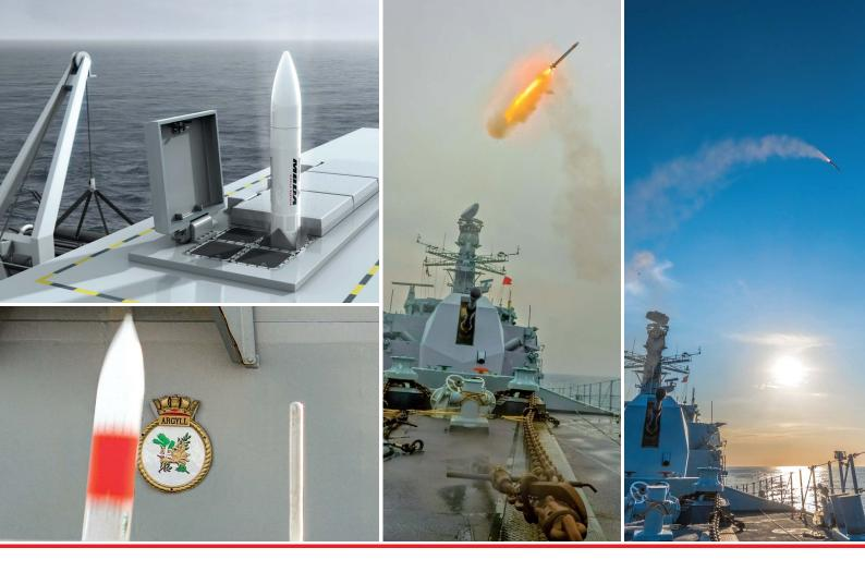
Sea Ceptor can be easily retrofitted into a wide range of platforms, ranging from 50 m OPVs to frigates and destroyers. Two main features provide this flexibility. Firstly, the use of 'soft-launch' weapon technology for a compact launch system that can easily be installed in a number of locations. Sea Ceptor can be targeted from the ship's existing surveillance radar and therefore does not require dedicated fire control radars.
