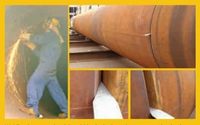
Welding is a central activity within the hydrocarbon construction business. Typical offshore structures involve fabrication of large tubular structures which are manufactured as per API2B standard. These tubular structures are further welded together based on various codes and standards, to form Piles and Jacket legs.
