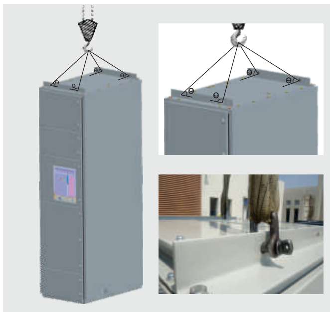
Figure 10 - Lifting angles
