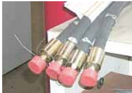
Hoses stored with both ends covered with plugs
