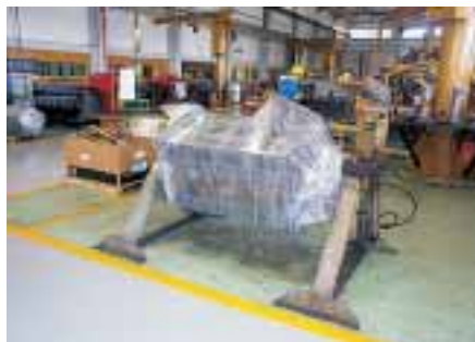
Components covered with plastic and stored
