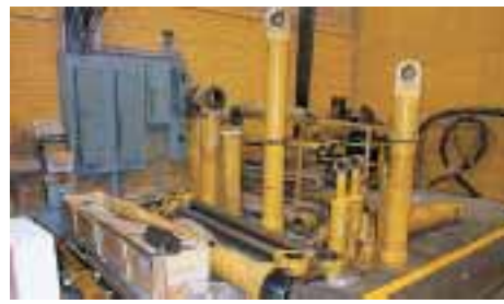
Cylinders not protected and not stored on racks
