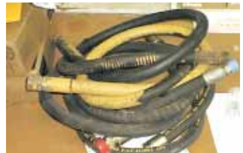
Hoses stored unprotected.
