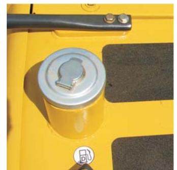
clogged, the pressure in the tank will drop and fuel will not flow freely to the engine. This hole should be cleaned from time to time.
