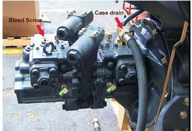
bleed plug. Hold the removed hose firmly, if possible higher than the oil level in the hydraulic tank, so that oil will not spill out of the hose. After bleeding is complete, first tighten the bleed plug and then install the hose. If the pump is run when the pump case is not full of oil, there will be abnormal generation of heat and this will lead to premature failure of the pump.
