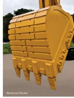
and increased wear plates enhance protection to the bucket. Lip guards between tooth-points and heavy duty tooth adaptors further extend the life of the bucket.
