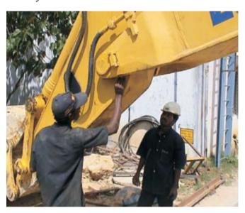
A well-kept machine at the site, excess grease being wiped after greasing
