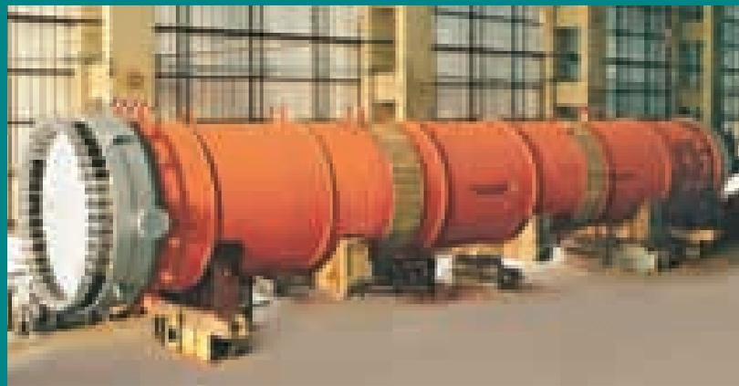
The world's largest ammonia converter for a fertiliser plant
