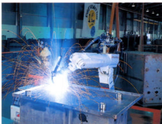
Robotic welding to ensure weld consistency.
