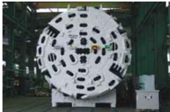
Tunnel boring machine at project site
