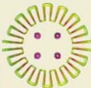
CFD results depicting contour of heat flux ( W/m^2 ) along tube wall
