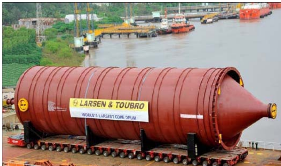
The coke drum at L&T's Hazira Works, ready for despatch.
