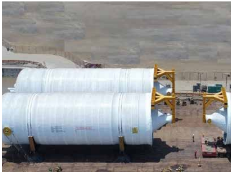
Coke Drums for Marathon Petroleum Corporation, USA
