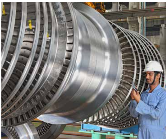
Supercritical turbine being manufactured at Hazira, Gujarat
