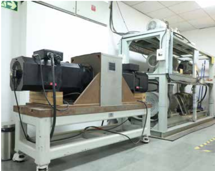
LTTS' Motor Dyne system conducts troubleshooting of power electronics
