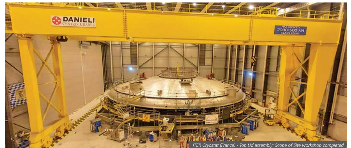
ITER Cryostat (France) - Top Lid assembly: Scope of Site workshop completed
