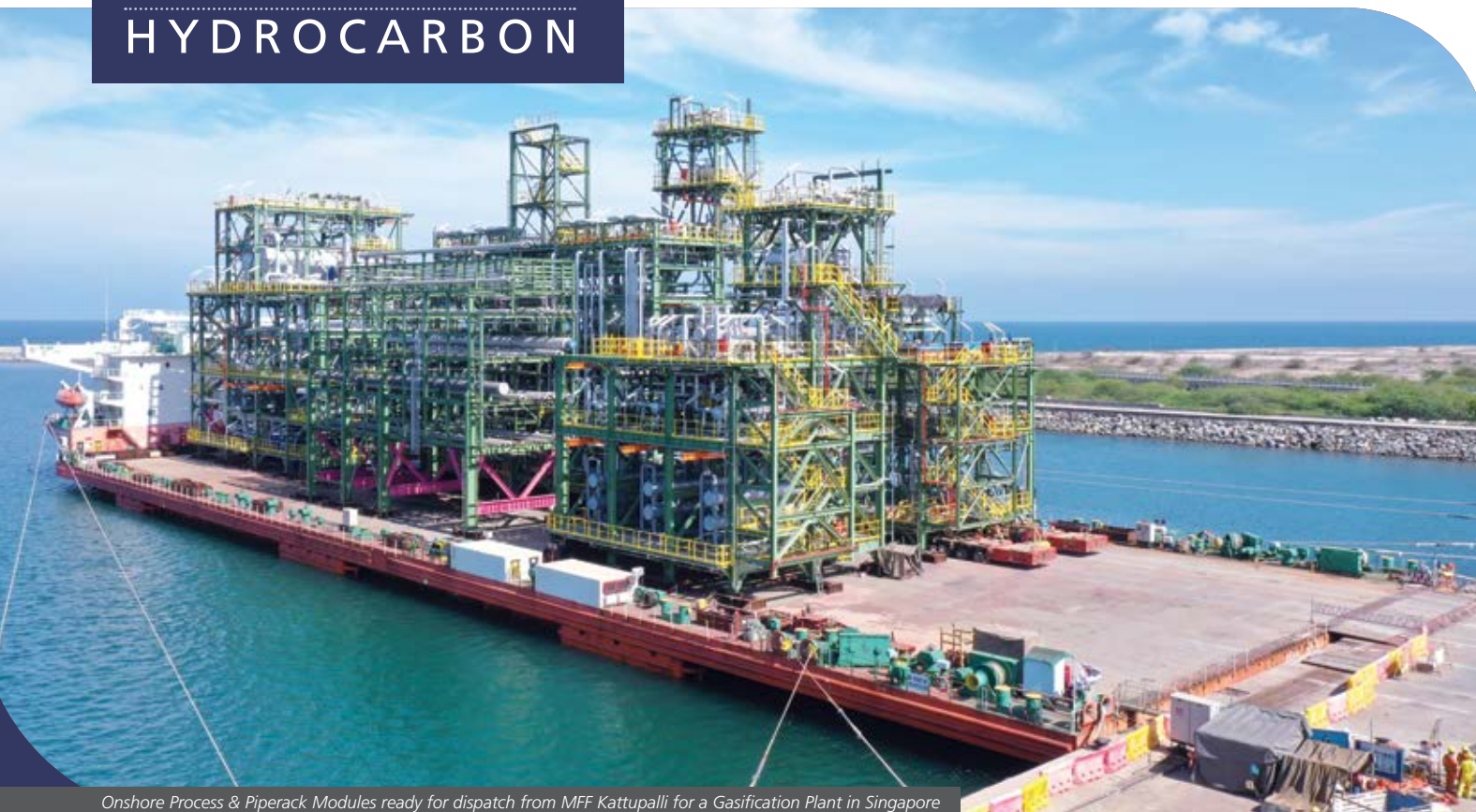
Onshore Process & Piperack Modules ready for dispatch from MFF Kattupalli for a Gasification Plant in Singapore
