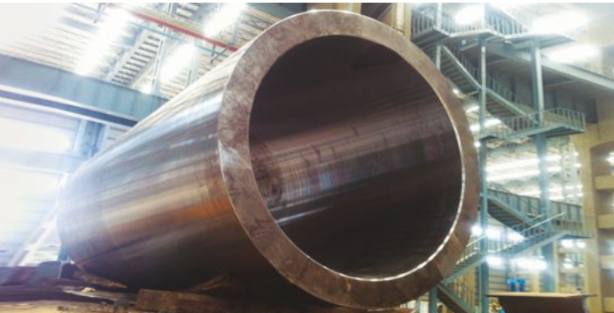
Forgings for Spent fuel Storage Casks MOC : SA 266M Gr2 Weight : 35 MT
