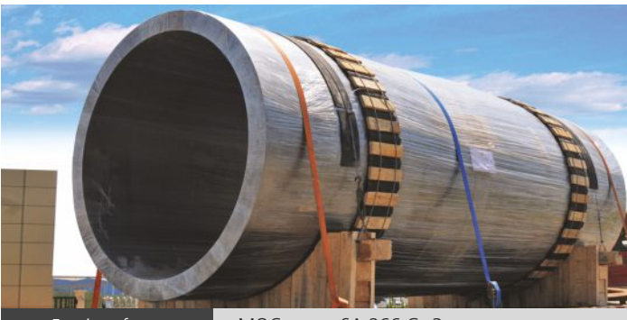
Forgings for nuclear project MOC : SA 266 Gr 3 Weight : 15 MT
