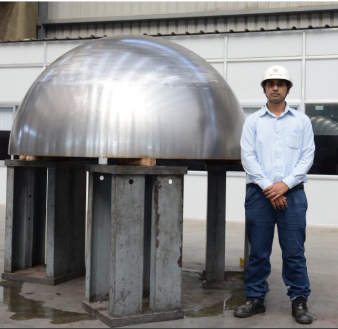
Formed torispherical head
