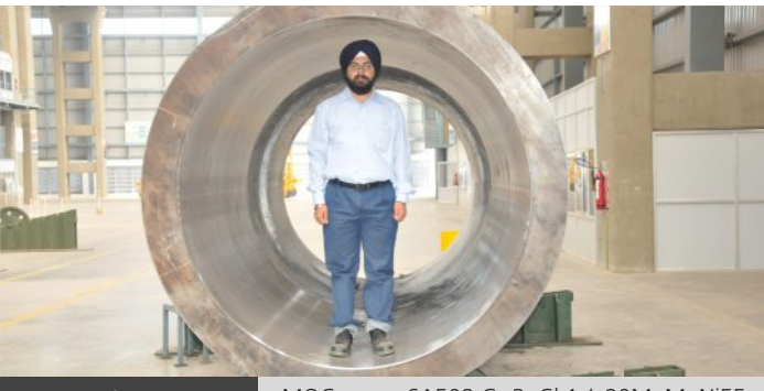
Forgings for Pressuriser Shells MOC : SA508 Gr 3 Cl 1 / 20MnMoNi55 Weight : 18 MT
