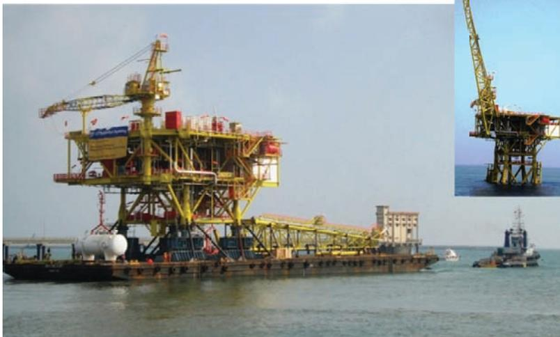
*Topside & Vent Boom being transported to Yetagun field (inset: Yetagun D Platform installed Offshore)*
