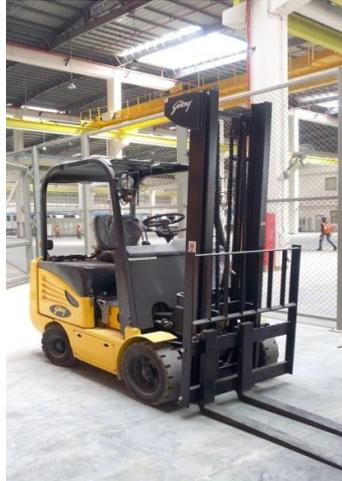
Fig-16:- Electric Forklift
