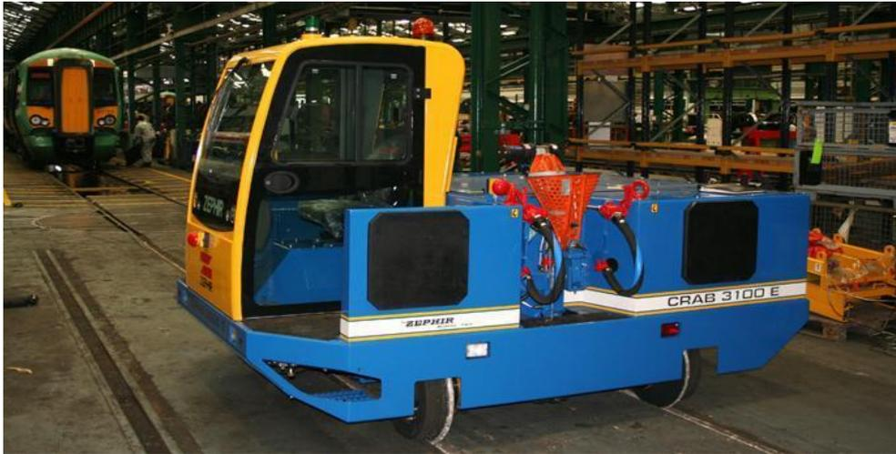
**Fig-11:- Battery Tractor**
