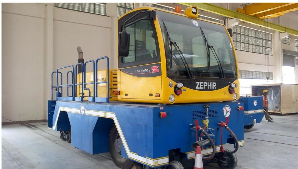
**Fig-12:- Diesel Shunter**
