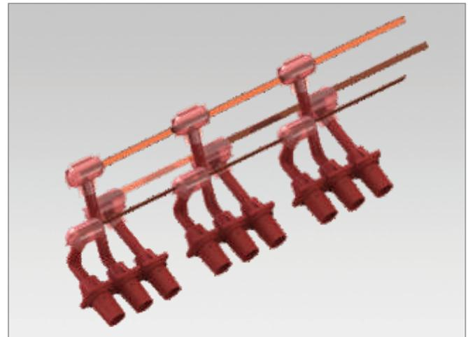
Figure 4.5.2 B Main Busbar Arrangement End Panel
